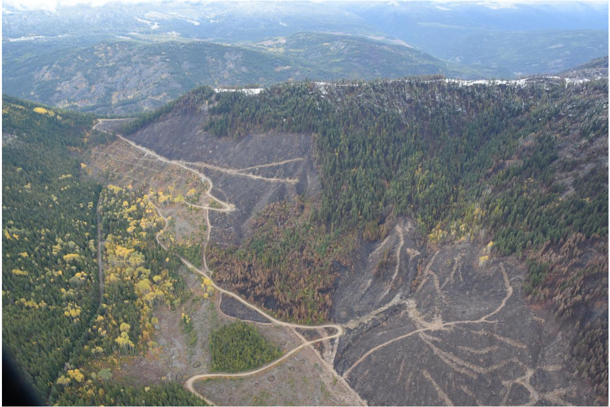
Photo 11. Bulldog Mountain fire. Looking west up Brooklyn Creek. Rail grade and entrance to Bulldog Tunnel are visible at left. Note landslide from road just above tunnel entrance. Cutblocks were logged in 2015 to 2016, and have unusually severe burn (mapped as “moderate” on BARC map).
